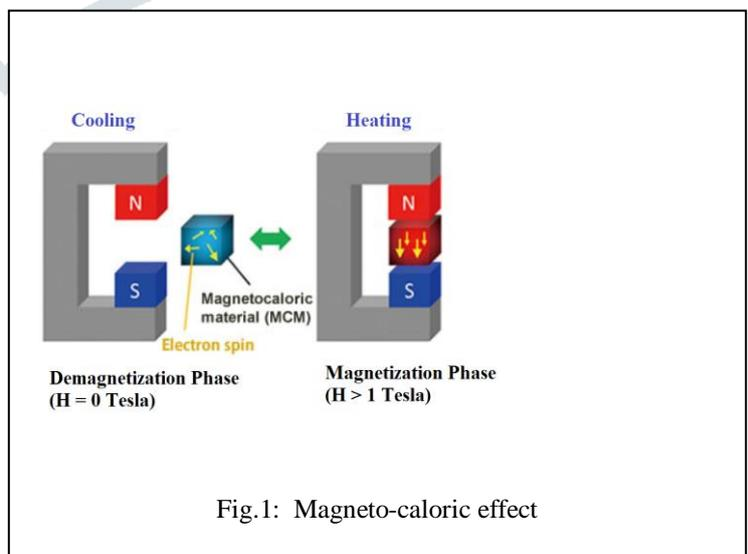
Fig.1: Magneto-caloric effect
