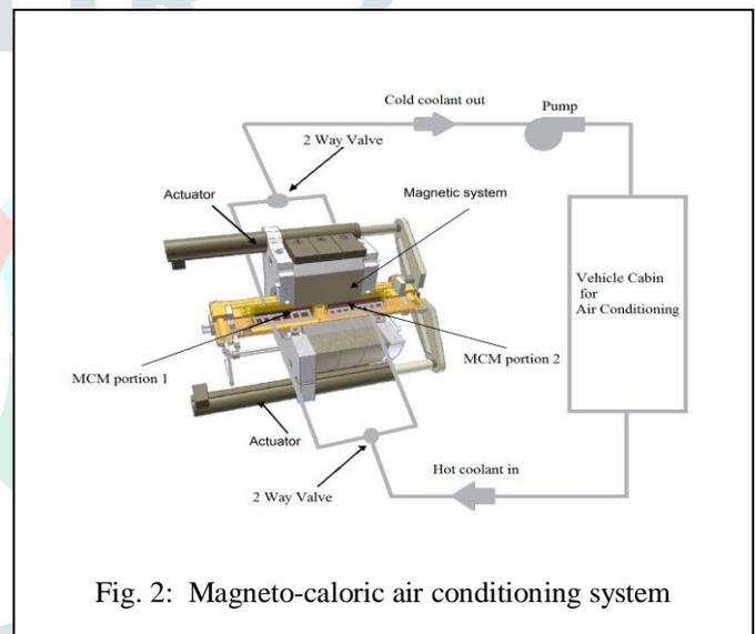
Fig. 2: Magneto-caloric air conditioning system
