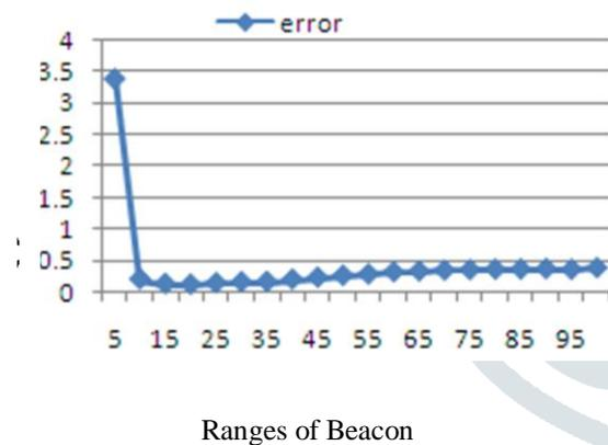
Fig.3.9 A graph between range of beacon and mean localization error
