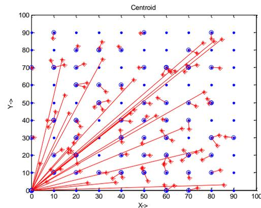
Fig 3.1 (A representation of 10m<sup>2</sup> grid size but radio range is only 5m of anchor )
