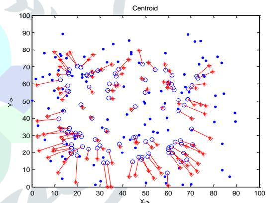
Fig.4.1 Random deployment of anchor nodes in 90x90 and testing nodes Within 80x80 working field.
