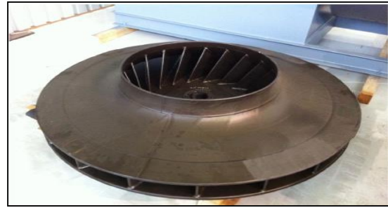
Fig 1.3: CS MOC impeller coated with Rubber lining on it.
