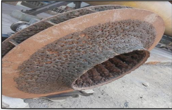
Fig 3.8: Deteriorated rubber lining on the Impeller
