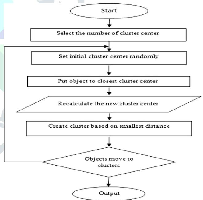
**Fig 2.1 K-Means Algorithm Flowchart**
