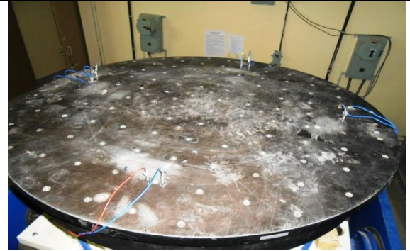
Figure8. Control and Monitor accelerometers at 450mm radius from the centre of the head expander
