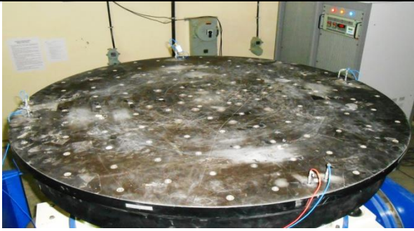
Figure6. Control and Monitor accelerometers at 550mm radius from centre of head expander
