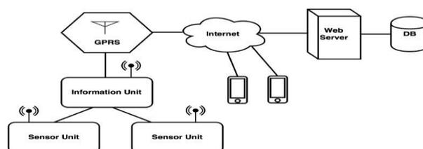
Fig. 2. System overview of automated irrigation system
