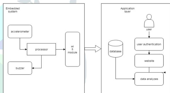
**Fig 1. Posture Detection System Architecture**
