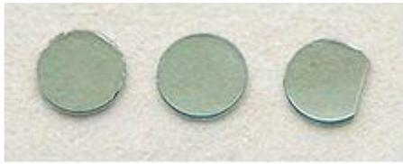
Fig 1. Synthetic SiC crystals (~3 mm in diameter)
