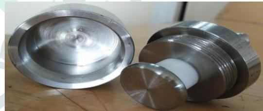
Fig.4(a) Open view of Stainless steel chamber & steel lid
