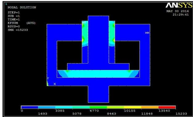
Fig. 5 Electric field pattern in Food cell
