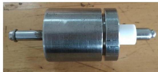
Fig.4(b) Closed view of Stainless steel chamber & steel lid as LV. The gap between the electrodes is adjusted to get a load impedance of 10  $\Omega$ . Resistance of the load circuit is given by conductivity, of milk is taken as 6 mS/cm [12], with  $R=10 \Omega$  and above values in equation (5),  $l=4.3$
