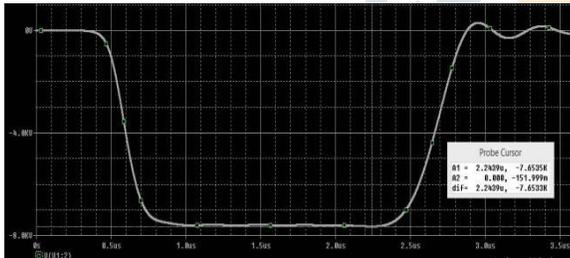
Fig.2 PSPICE voltage waveform of Type-B PFN
