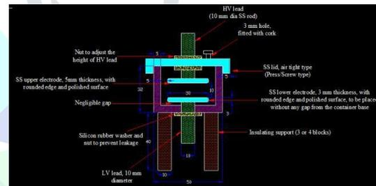
Fig.3 Diagram of Food processing chamber
