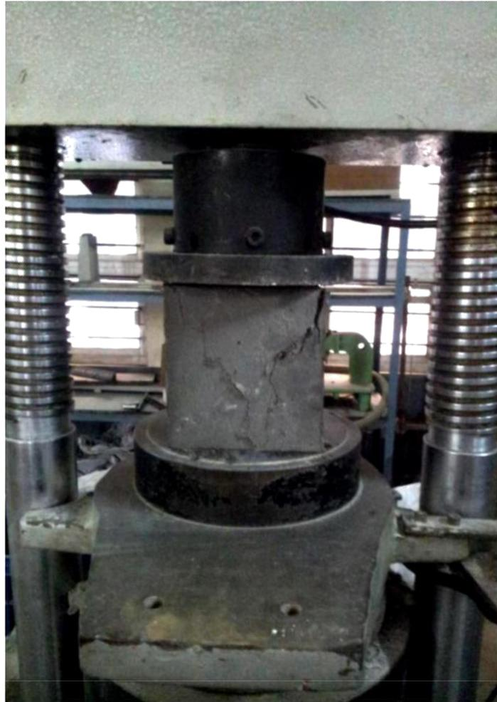
**Figure: Concrete cube subjected to compression**
