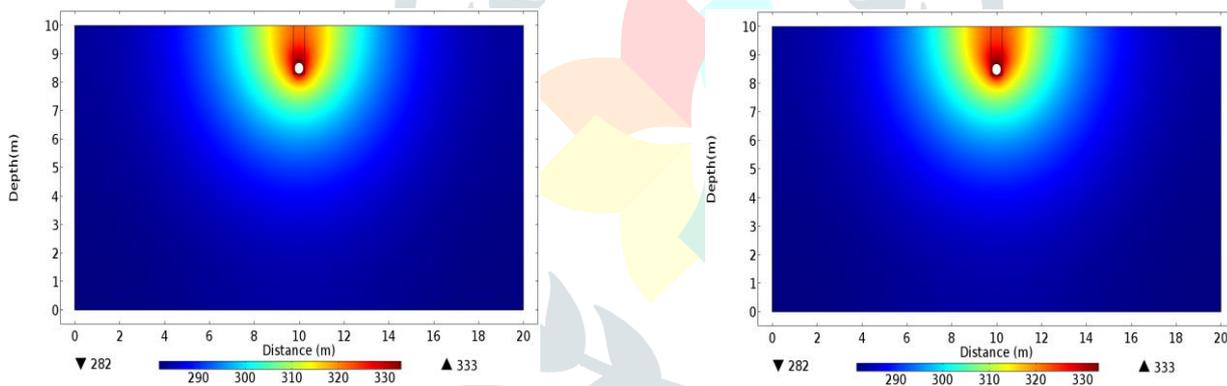
Figure 6: Temperature rise above the cable at 0.2 m depth from the surface considering low thermal conductivity of 2.0 W/m.K (native material) after 5 days a) without natural convection b) with natural convection.
