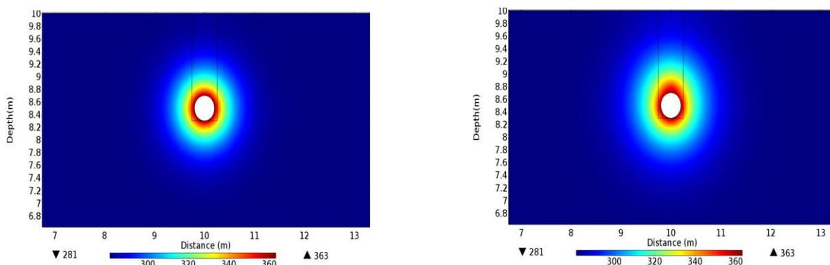
W/m.K (trench backfill material) after 5 days a) without natural convection b) with natural convection.
