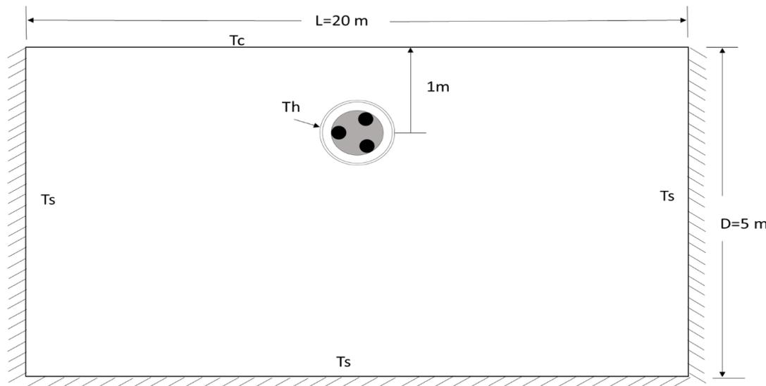
Figure 4: showing temperature and flow boundary condition. No flow is allowed from system to the surrounding.
