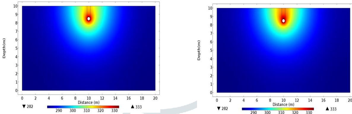
Figure 5: Evolution of temperature field after 365 days around the cable. a) Only conduction b) with natural convection  $K=10^{-9}m^2$  c) with natural convection  $K=10^{-8}m^2$  d) with natural convection  $K=10^{-7}m^2$
