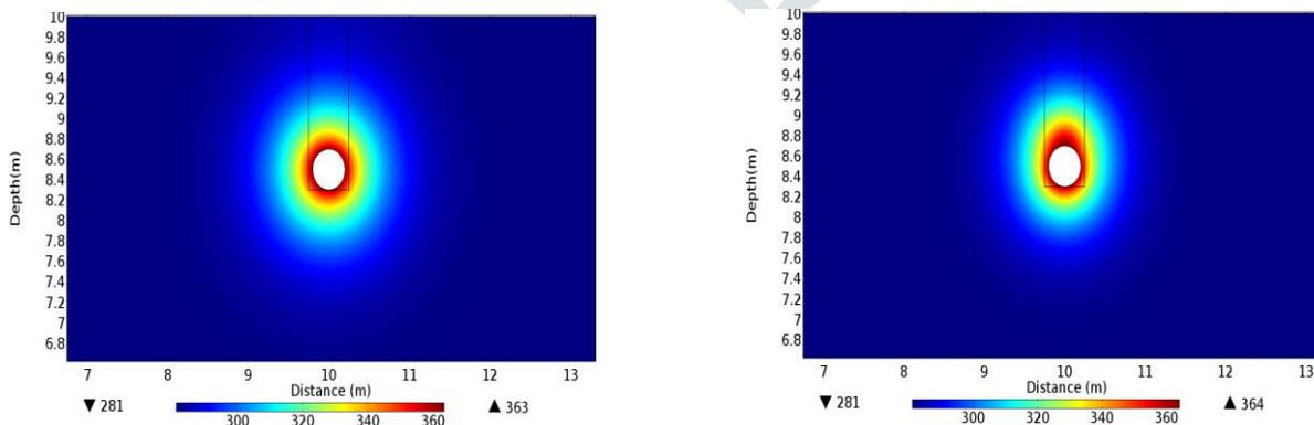
Figure 7: Temperature rise above the cable at 0.2 m depth from the surface considering high thermal conductivity of 3.5
