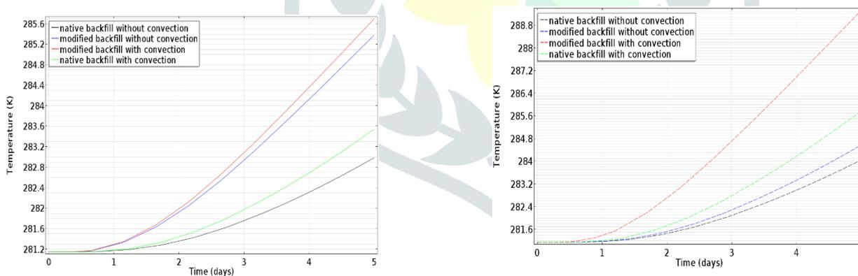
Figure 9: Temperature rise above the cable at 0.2m depth after 5 days a) in native soil b) with modified trench backfill.
