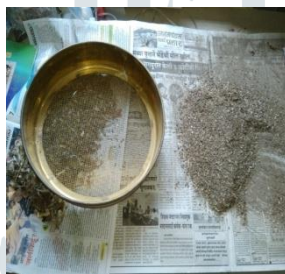
Plate 3.17 : Grinding and Screening of solid waste in 2mm sieve.
