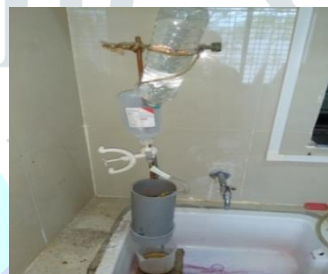
3.18: Leachate preparation assembly and collection in beaker
