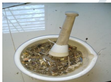
Plate 3.17 : Grinding and Screening of solid waste in 2mm sieve.
