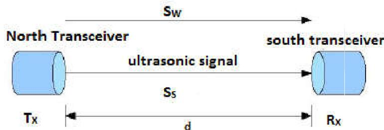
Figure:- Ultrasonic Sensors arrangements
