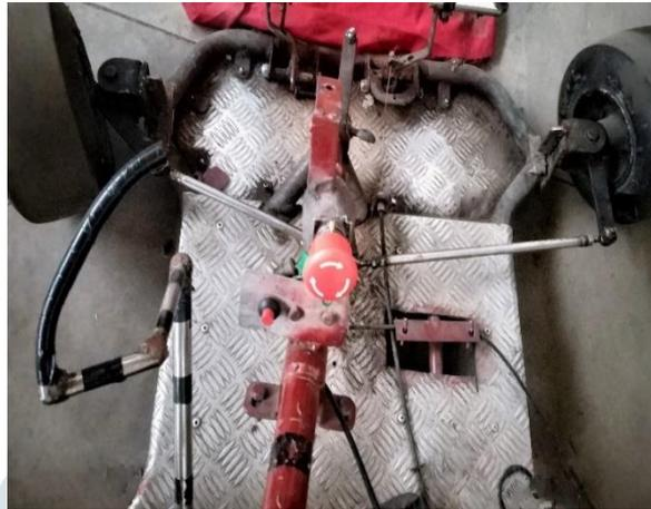
**Fig. 6.** Steering system from driver's point of view.
