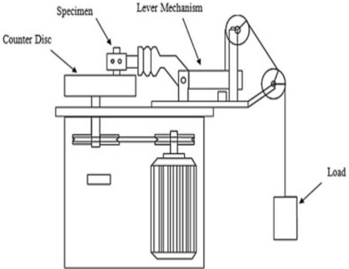
Figure3.1:Schematic diagram of Pin on Disc Test Setup
