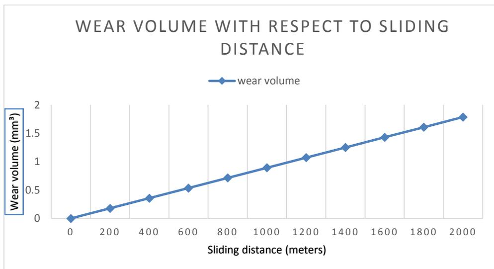
Figure4.1:Wear volume v/s sliding distance in experiment no.1
