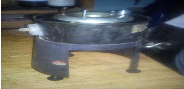
**Fig 1: Redwood viscometer for the measurement of Kinematic viscosity**
