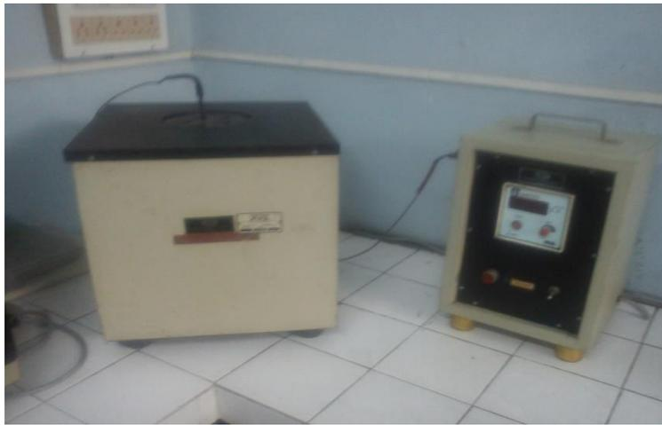
**Fig 6: Carbon Residue (Rams Bottom)**
