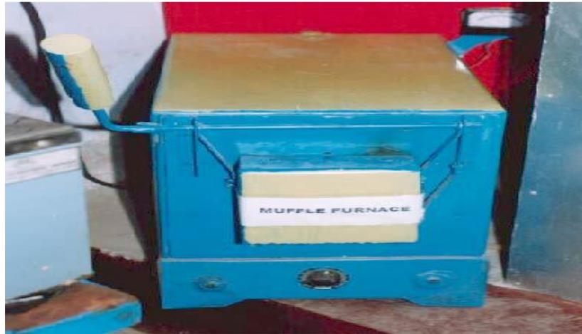
**Fig5: Muffle furnace for of ash content**
