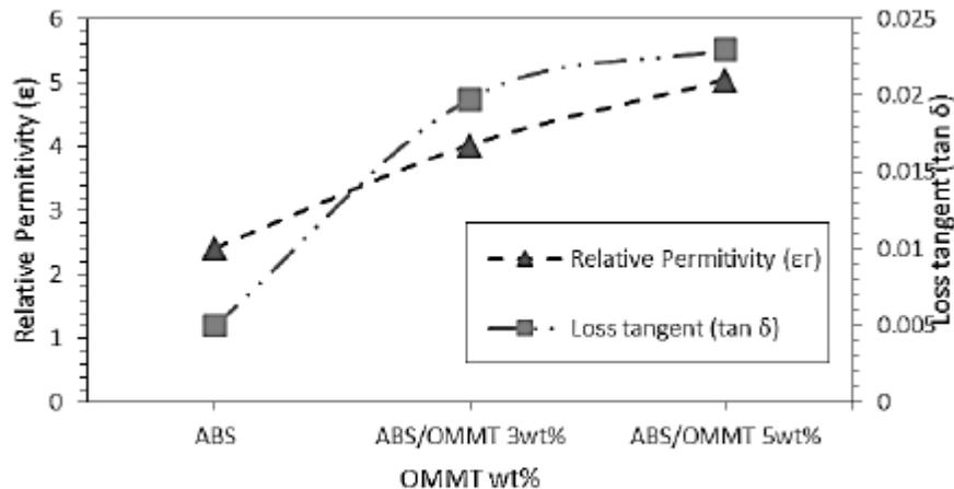
Figure 3 relative permittivity and loss tangent
