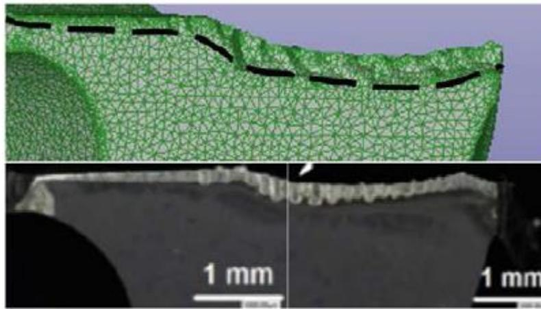
**Fig. 8:** Cutting tool showing wear rate [11].
