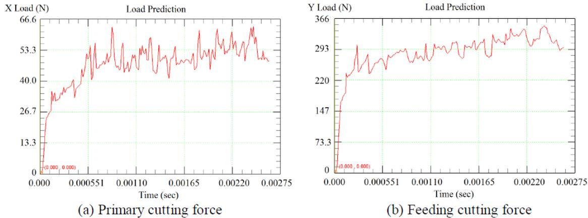
**Fig. 4:** Graph of cutting force with parameter [9].
