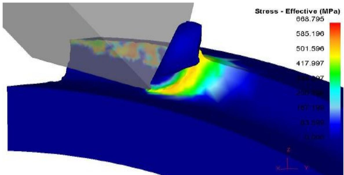
**Fig. 3:** Stress contour in front cutting edge [9].
