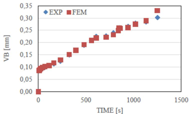
**Fig. 9:** Comparison of experimental and simulation wear rate [11].
