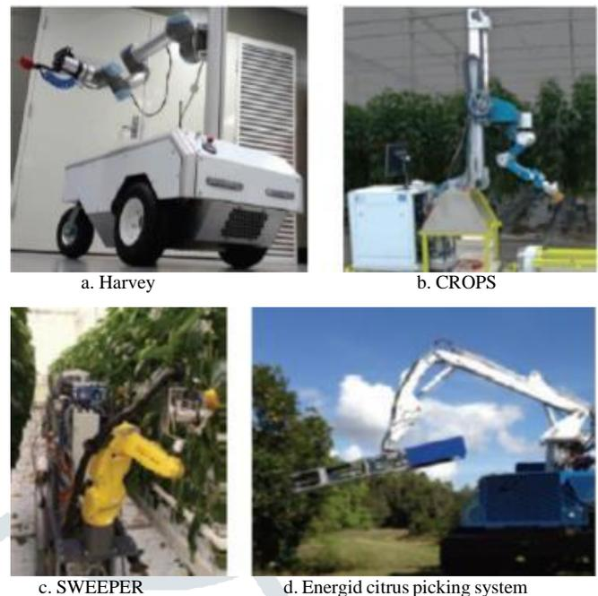
Fig 5. Harvesting robots[14]
