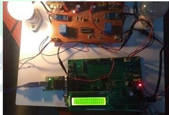
Fig-4: kit in operating condition gives values of voltage & current
