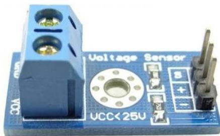
Fig3. Voltage Sensor
