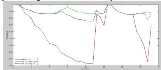
Fig. 2 comparison of voltage profile at each bus without and with DG placement using GA and PSO.
