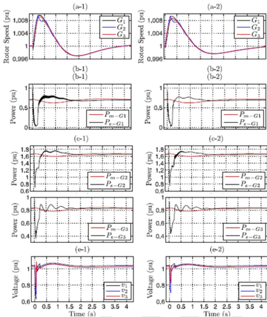
Fig. 11. Responses of the nine-bus system without RFCL (left column) and with the RFCL in line L45 (right column). (a) Generators rotor speeds. (b)–(d) Electrical and mechanical powers of the generators. (e) Generators terminal voltages.
