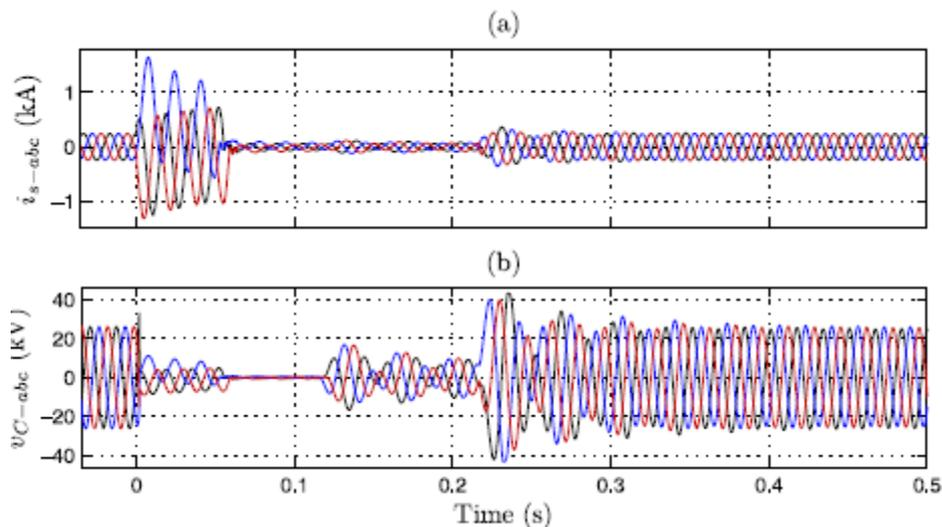
Fig. 10. Responses of the nine-bus system subsequent to the strike of fault Flta . (a) Line currents. (b) Capacitor voltages.
