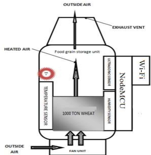
**NodeMCU:** It is a microcontroller that to which the sensors DHT11 and ultrasonic HC-SR04 are connected. It also has Wi-Fi module in it, with which the values sensed by sensors are sent through.
