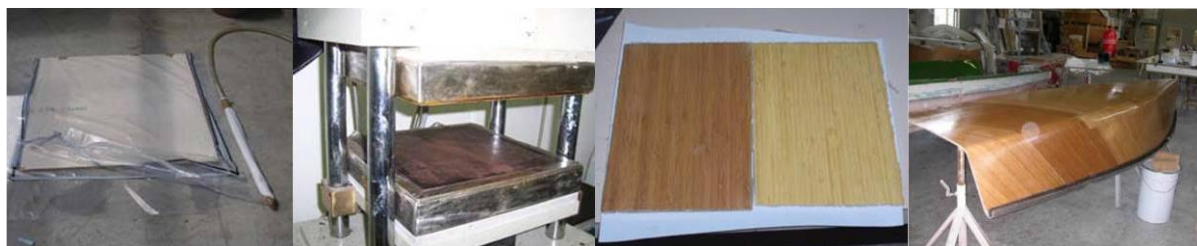
Figure 6. Fabrication of bamboo boat hull[34]
