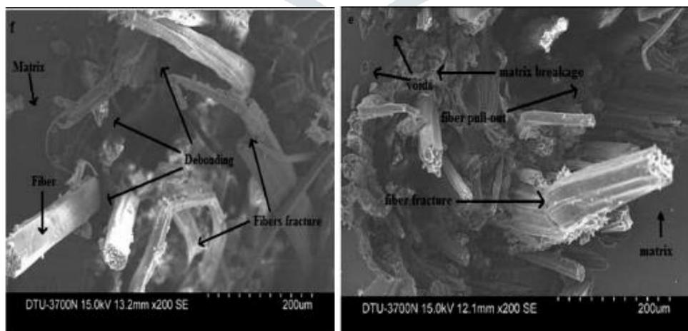
Figure 5 SEM image of a) jute/hemp/flax reinforced epoxy composites b) Hemp/Flax/Epoxy Composite [7]
