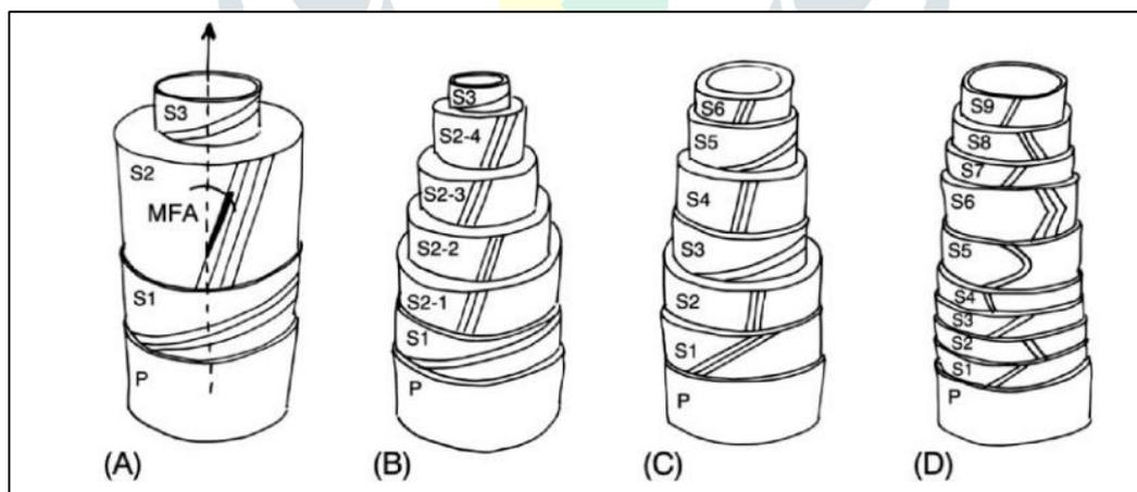
Figure 2 Schematics of possible cell wall organisation in (A) wood fibres, (B) bast fibres, (C) plant fibres and (D) seed fibres. Black lines indicate orientation of cellulose microfibrils.
