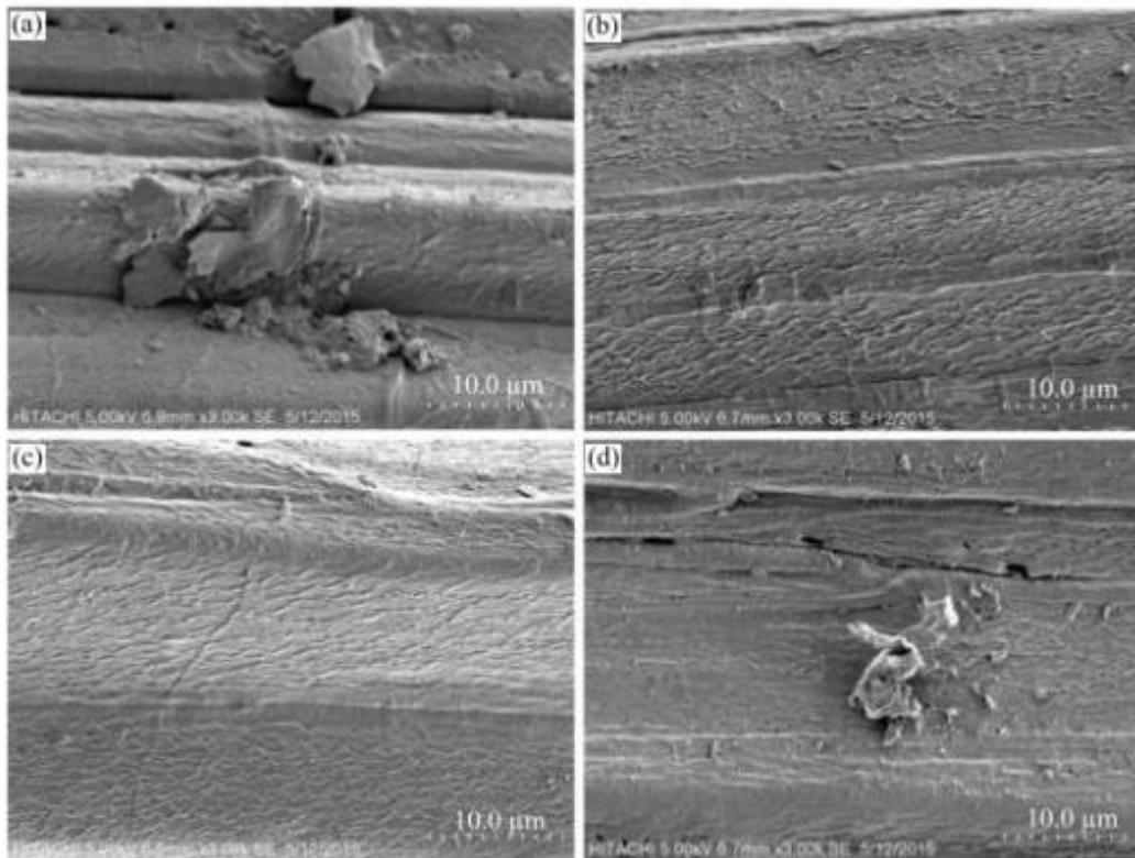
Figure 4a SEM of (a) untreated, (b) Alkali solution, (c) Silane and (d) Alkali-Silane treated Kenaf fiber[6]
