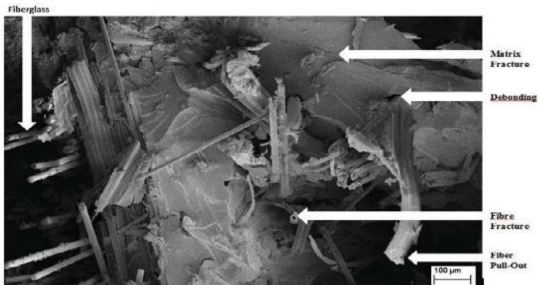
Figure 6 shows the SEM images of fractured bio composites [15]
