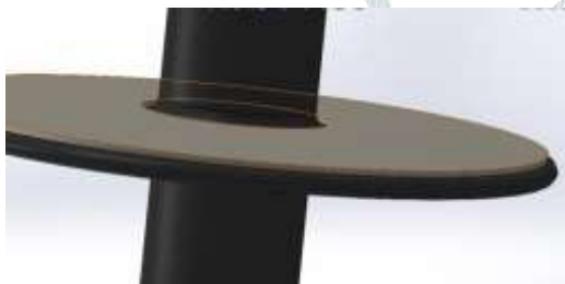
Fig 17: Dust Deposition of 1mm on each Disc
