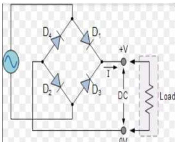
Fig.2 Rectifier circuit
