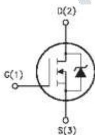
Fig .8 Internal schematic Diagram of MOSFET
