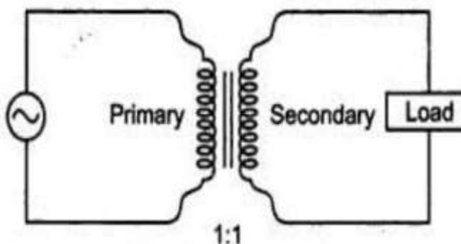
Fig.4 Isolation transformer
