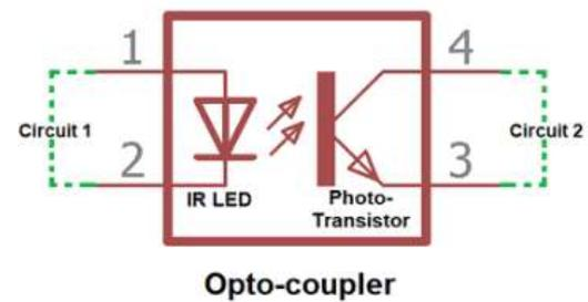
Fig.13 Design of Optocoupler
