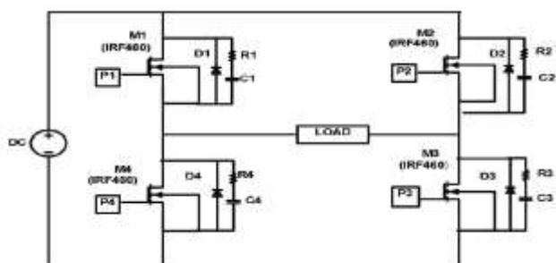
Fig. 3 DC-AC CONVERTER
