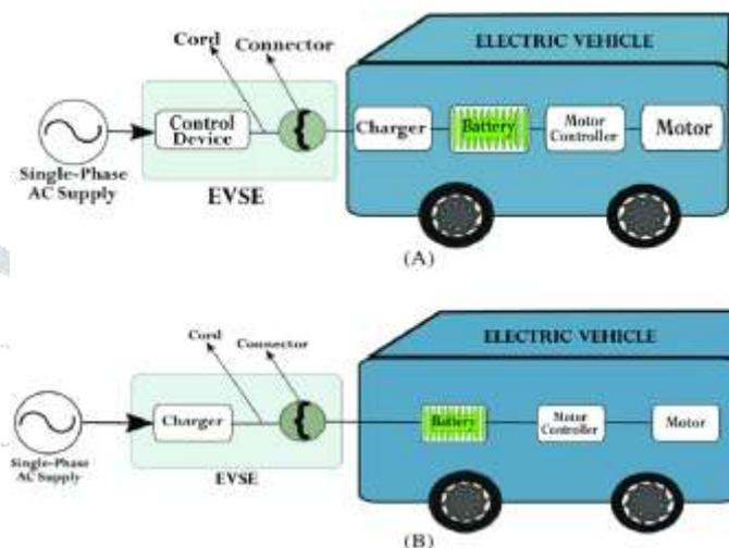
Fig. 1 (A) On board charger (B) OFF board Charger
