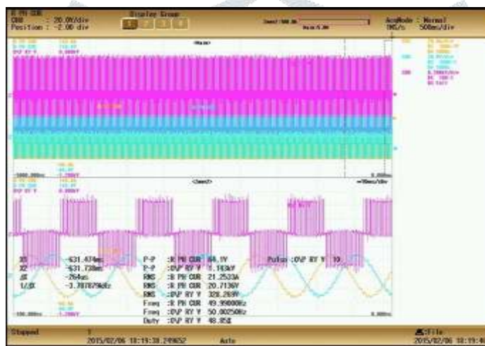
Fig. 8: V/f control at 50Hz with 25HP motor
