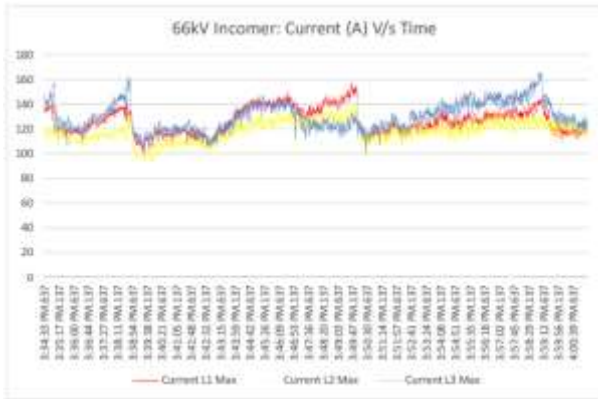
Graph 2 : Current trend chart on 66 kV bus for stabilised operating condition of plant
