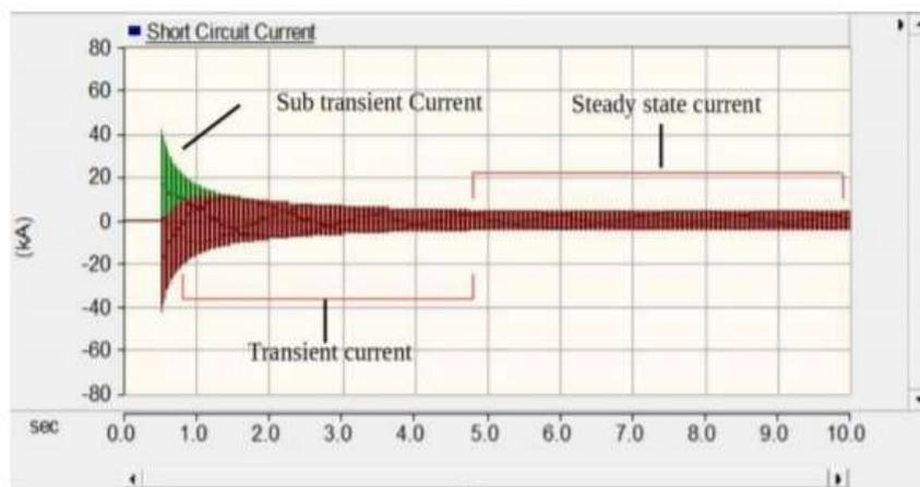
Fig. 6. Short circuit current of a 4-Pole Machine
