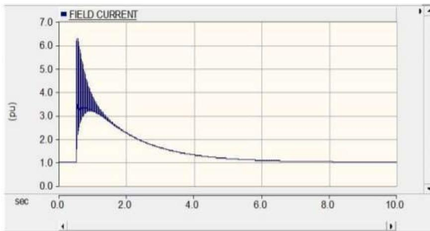
Fig. 5. Field current of a 4-Pole Machine
