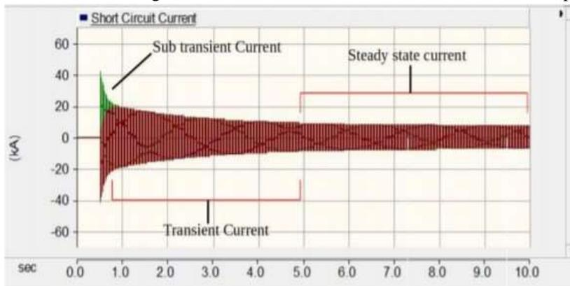
Fig. 8. Short circuit current of Salient Pole Generator.
