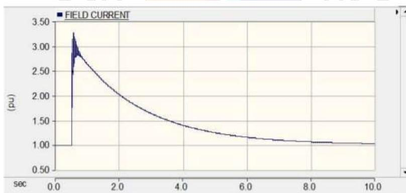
Fig. 7. Field current of Salient Pole Generator with Dampers
