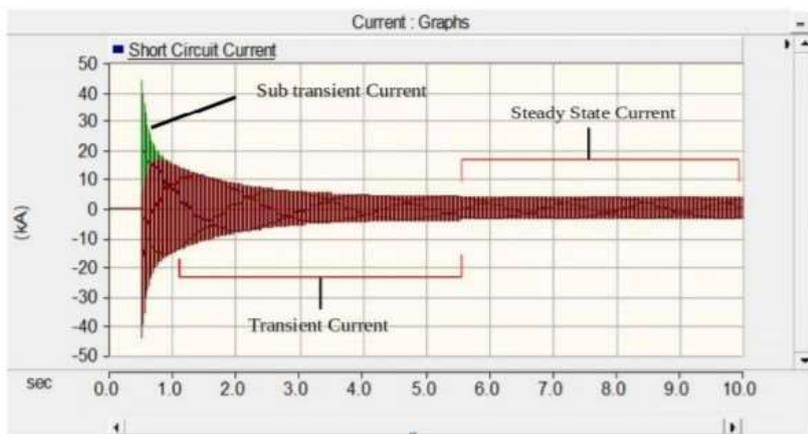
Fig. 4. Short circuit current of a 2-Pole Machine
