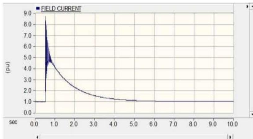
Fig. 3. Field current of a 2-Pole Machine
