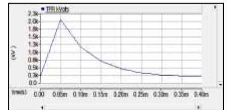
Fig. 9. Voltage at the transformer
