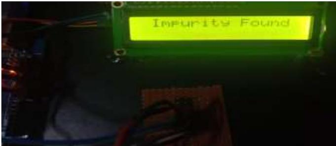
Fig.6. LCD display for alcohol and smoke detection system
