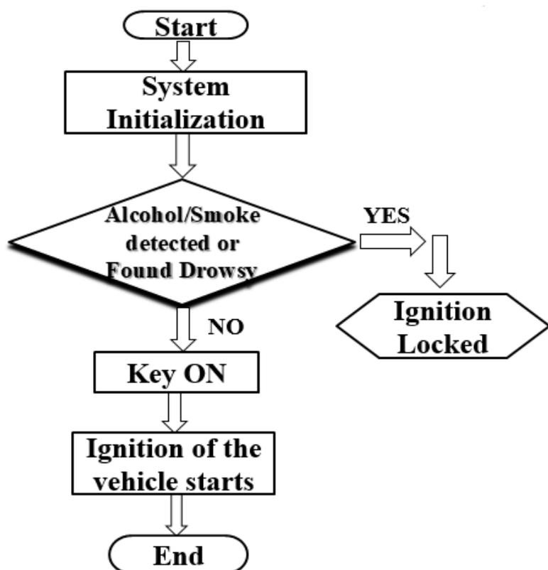
Fig.5. Flow Chart of the Process
