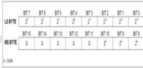
Fig: DS18B20 Temperature sensor register format.
