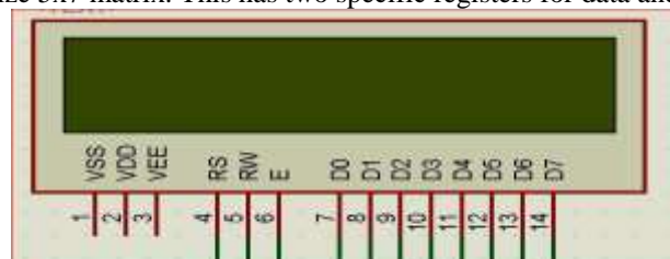
Figure 3.1: 16x2 LCD module
