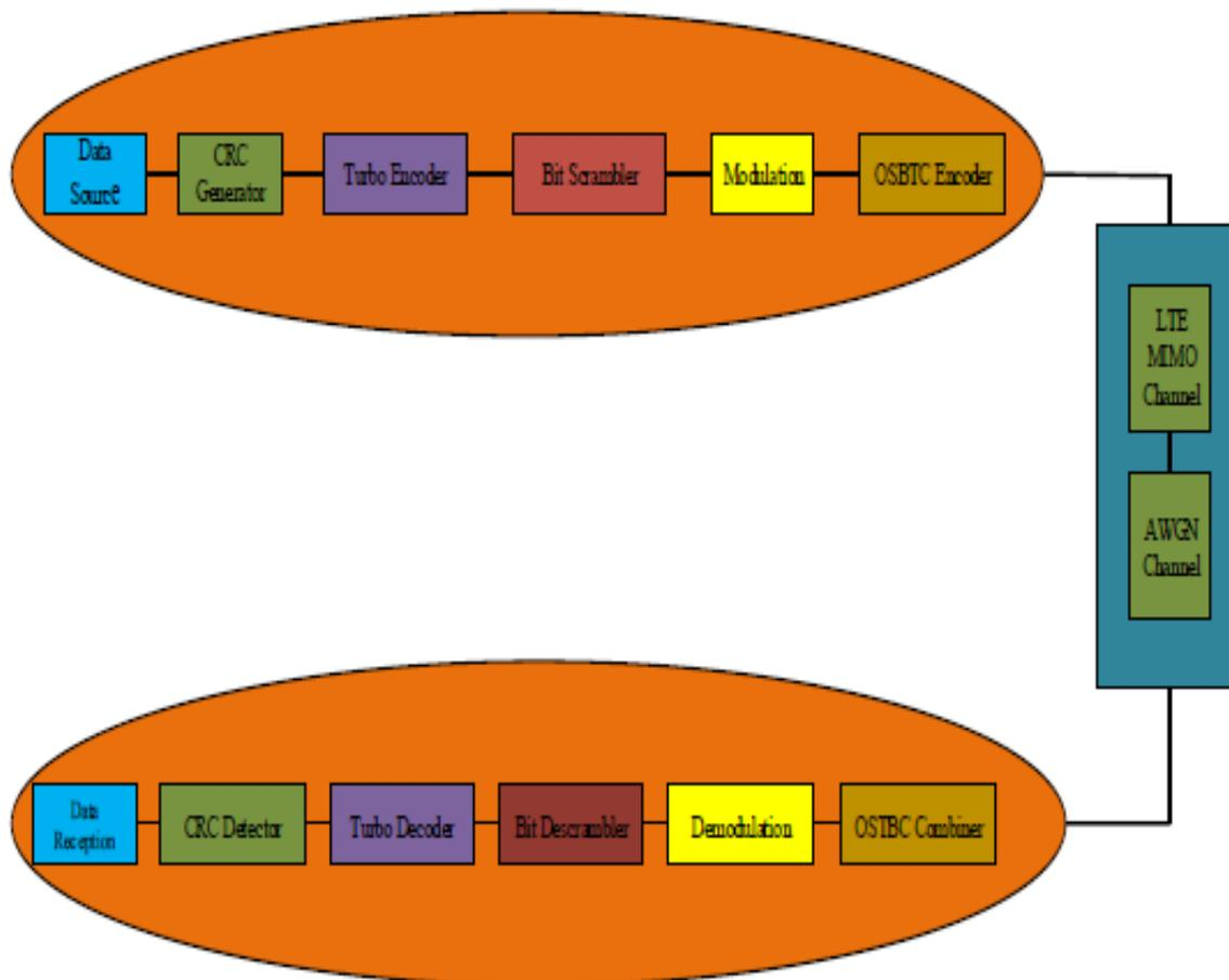
Fig.1 DL-SCH AND PDSCH Channel Model
