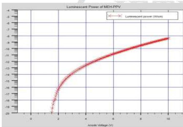
**Fig. 3. Luminescent power with respect to the anode voltage.**
