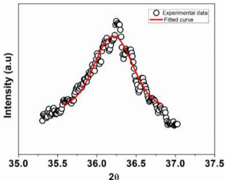
**Figure 2:** Calculation of full width at half maxima (FWHM) by Gaussian fitting of the (101) peak
