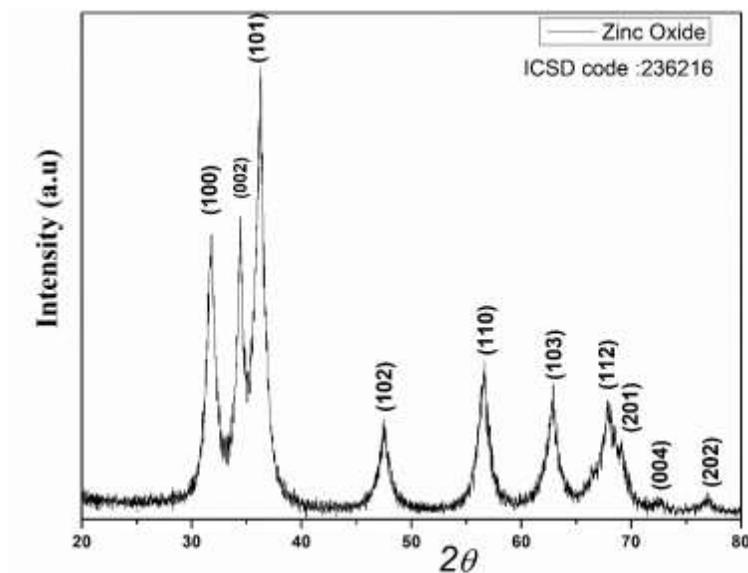
**Figure 1:** X-ray diffraction pattern of the undoped zinc oxide nanostructures
