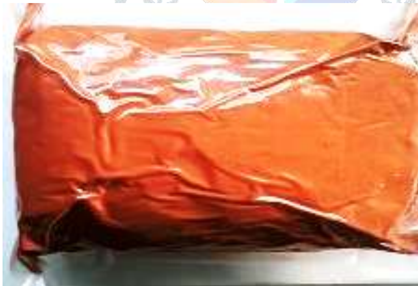
Fig 10. Cuprous oxide nano powder Cuprous oxide grinding powder 100-150 Nano particle size
