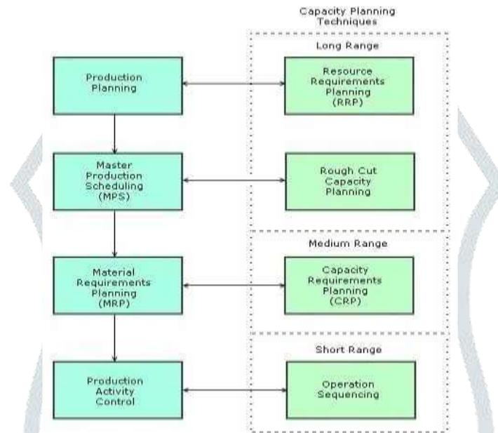
Fig.4 : Capacity Planning Technique
