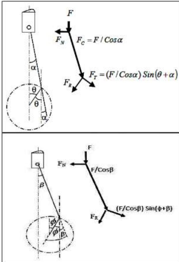
In the above figure,  $F$  represents the force exerted on the piston due to gaseous pressure.  $\alpha$  and  $\theta$  represent the inclination of connecting rod to the line of motion of piston in conventional and offset IC engine respectively,  $\beta$  and  $\phi$
