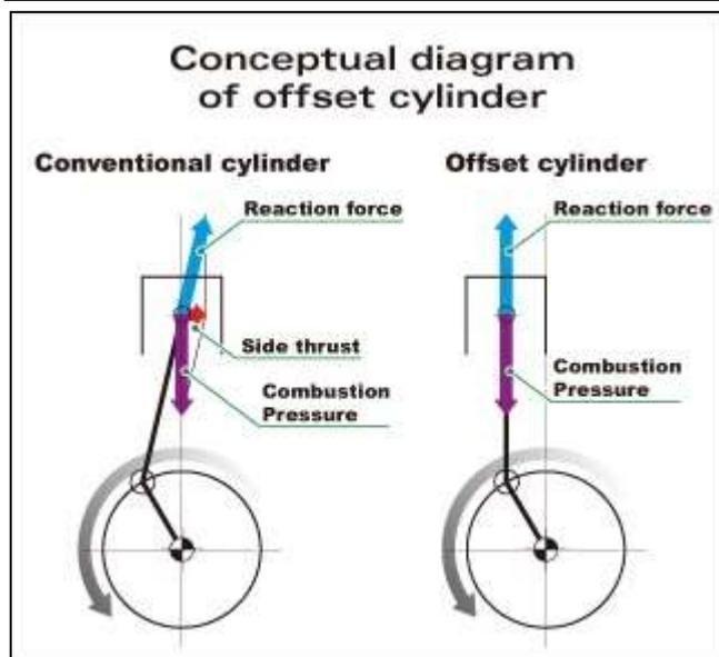
comparison of inline, offset, and twin crankshaft engine and P. Ragot & M. Rebbert for the influence of crankshaft offset on piston friction.
