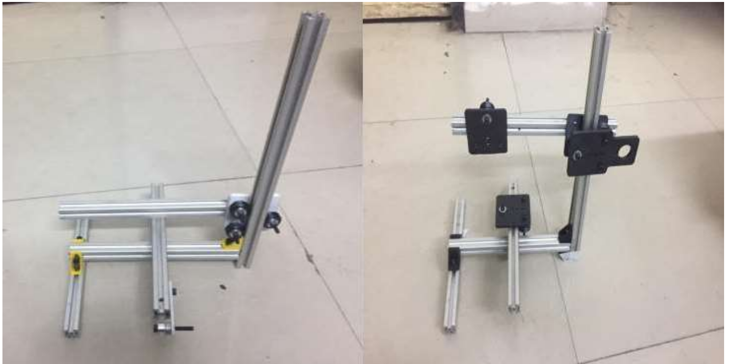
Figure 3 Structure for the deposition system
