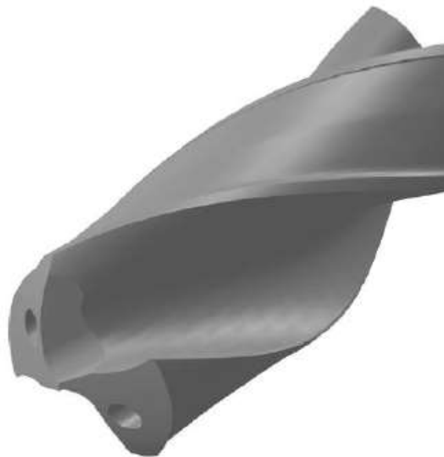
Fig. 5: 3D Modeling of drill tool [10].
