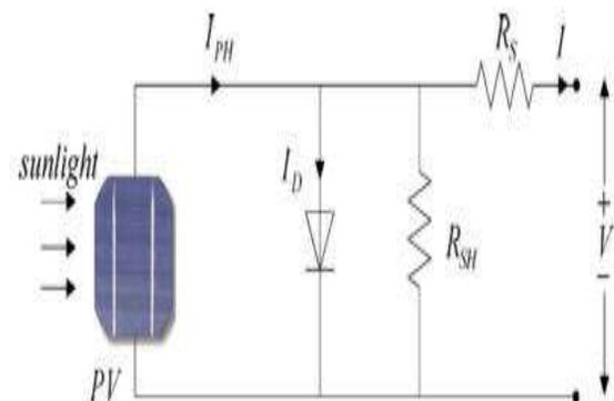
Fig. 1: Equivalent circuit of solar cell [8].
