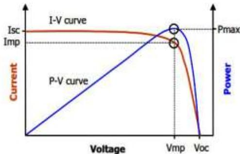
Fig.2: Shows the I-V and P-V characteristics of an ideal solar cell [6-8] whose equivalent circuit is shown in Fig.1 having a source of current ( $I_{ph}$ ), a diode with internal shunt resistance ( $R_{SH}$ ), an internal series resistance ( $R_S$ )
