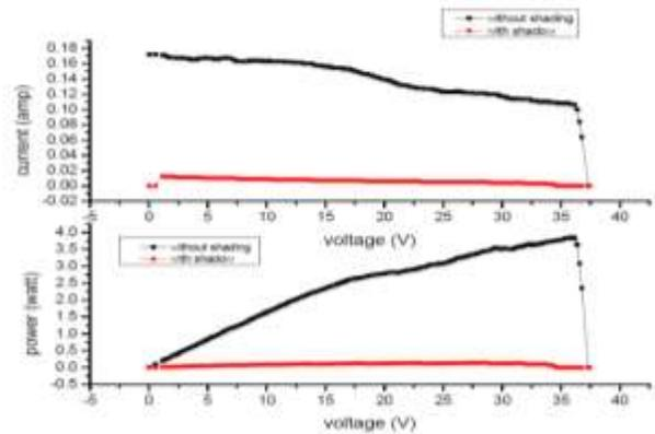
Fig. 6: I-V and P-V characteristics of test bench PV modules connected in series without Bypass diode under different shading profile.
