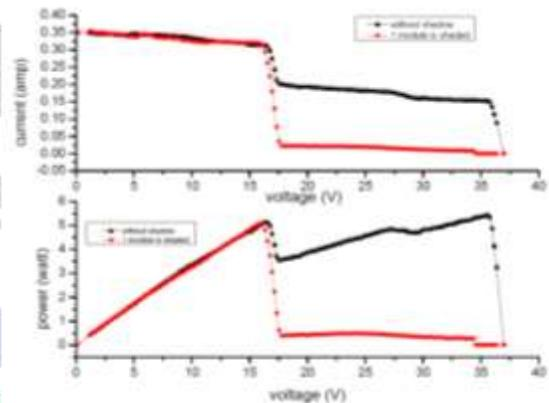
Fig. 7: I-V and P-V characteristics of test bench PV modules connected in series with bypass diode across each module, under different shading profile.
