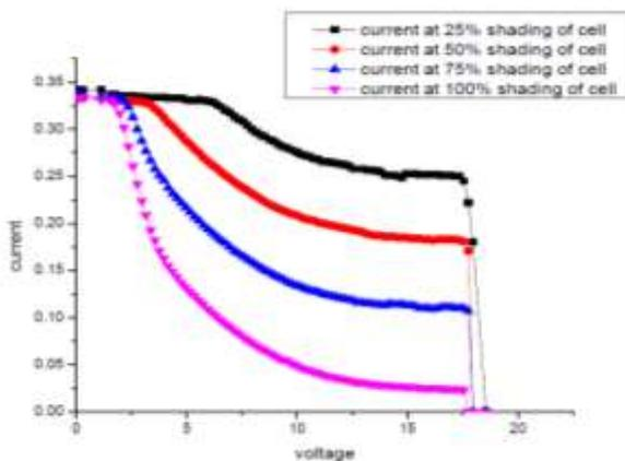
Fig.4: Effect of shading at cell level without bypass diode
