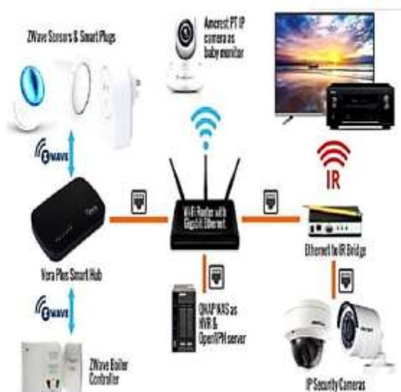
Figure. 6. The Z-Wave Network
