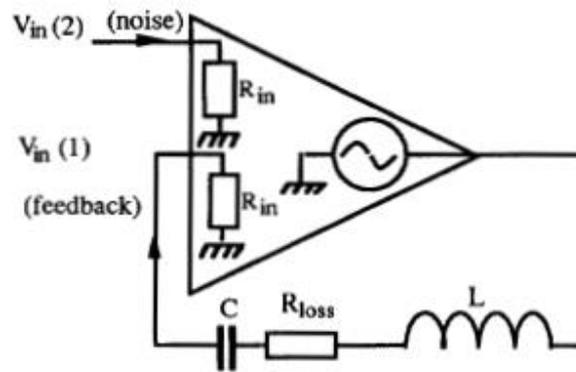
Figure 1. Equivalent circuit model of oscillator
