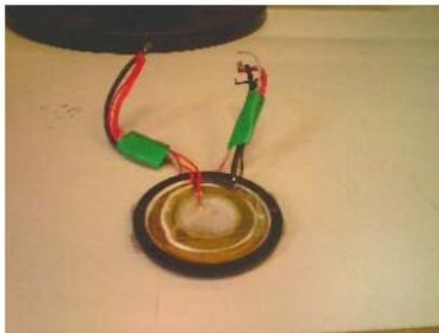
Fig 1: A stack of four piezo discs connected in parallel (see online version for colors)
