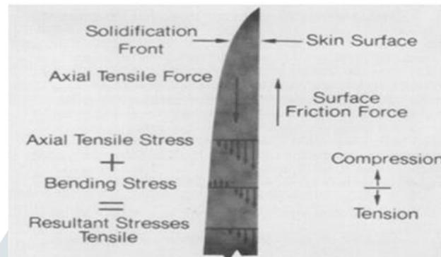
**Fig. 2 Schematic Drawing Of Axial And Bending Stresses In The Solid Shell Resulting From Friction In The Mold**
