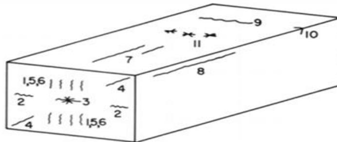
**Fig. 1 Schematic drawing of casting showing different cracks**
