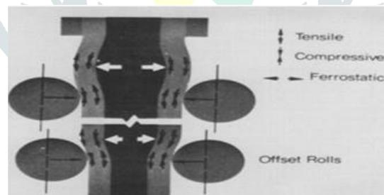
**Fig. 3 Axial stresses in the solid shell**
