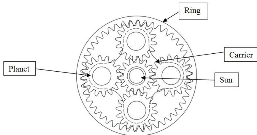
**Figure 1: Schematic diagram of a planetary gear train**
