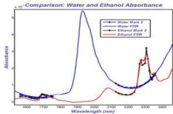
Figure 5. Mark 2 Measurement performance comparison compared to FTIR.
