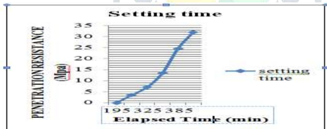
INITIAL SETTING TIME CORRESPONDING TO 3.5 MPA RESISTANCE - 290 MIN
