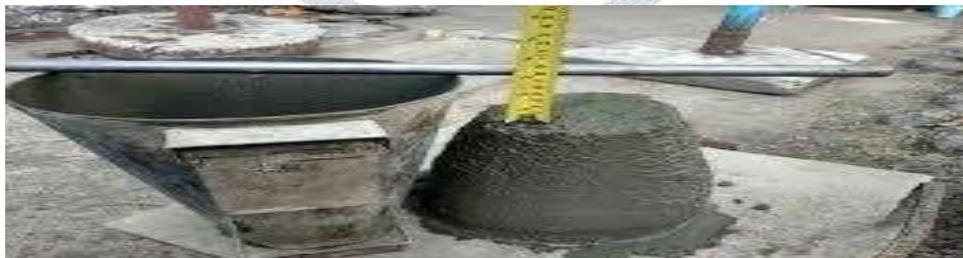
**SLUMP CONE TEST OF CONVENTIONAL**
