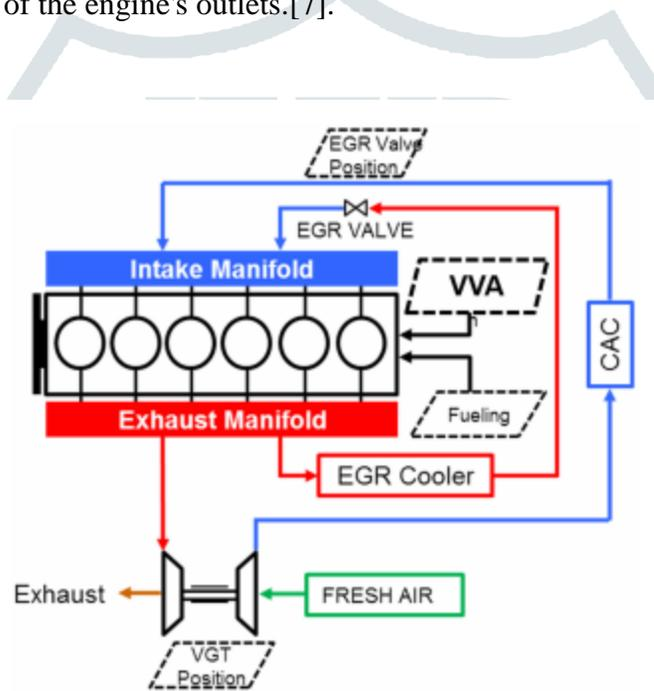
**Figure 1: Illustrating the Schematic for the Experimental Test-Bed Engine**
