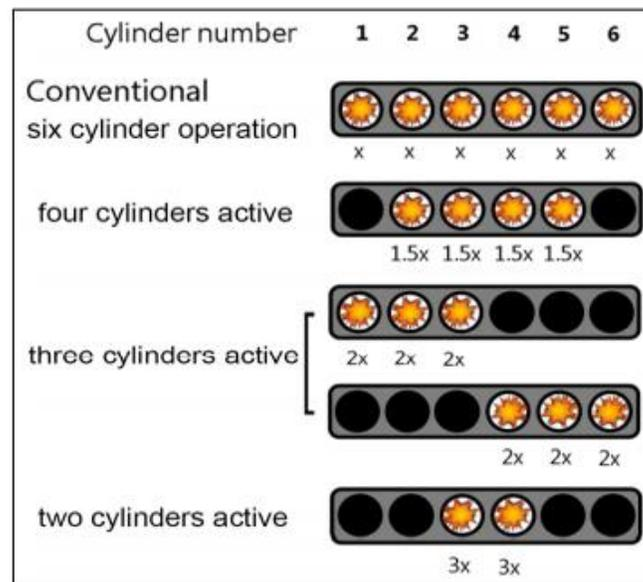
**Figure 2: Active Cylinder of the Different Mode of the CDA, Alongwith the Distributions of the Fuels to Each of the Cylinders Assuming Tool Fuels of the '6x' needed for Sustaining Certain Loads**
